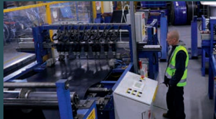
Elevator belts being slit and punched to order PLC controlled belt slitting and punching operations
